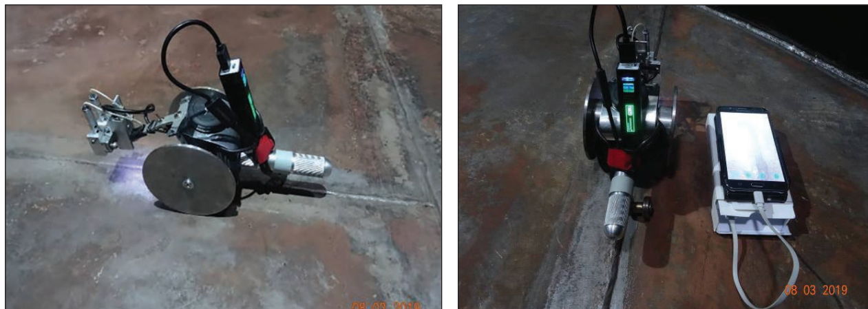
Figure 5. Testing of the VK/TVA-1 visual information recording device on the welded joints at the bottom of the VST-200 tank
