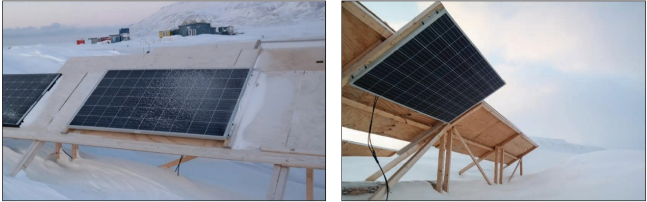
Figure 3. Module installation with a sky-facing module (left) and a ground-facing module (right). The modules are lifted 2 cm from the wooden surface to allow for ventilation (Frimannslund et al., 2021)
